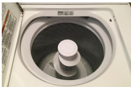
Figure 2: The central agitator in top-loading washing machines is thought to contribute to higher microfiber releases compared to front-loading washing machines.
